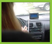
In Oregon, onboard units used GPS technology to record mileage driven in specific zones.
