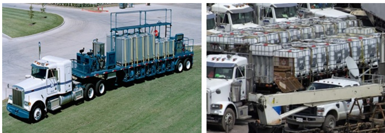
Figure 5-7. Metal and high-density polyethylene (HDPE) chemical additive units.
