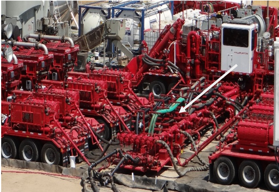
Figure 5-9. Manifold (pointed to by the white arrow).
